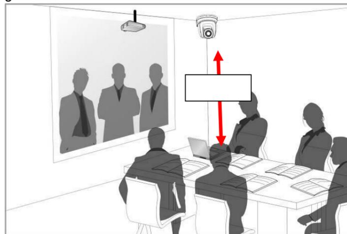
3. The camera (including metal plates) weights approximately 2.5 kg. If it is to be installed on the ceiling, please use the hanger that has obtained UL security approval to prevent the camera from coming loose and falling.
