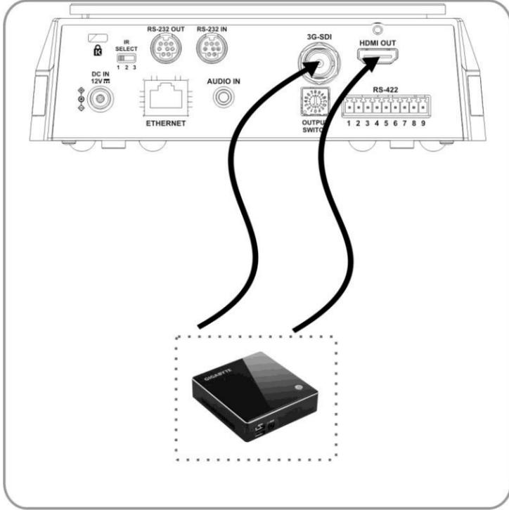
4.3.2 Connecting to an HDTV/computer monitor via HDMI
