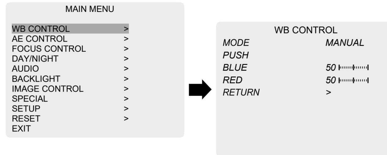
1. Adjust White Balance first by using the AWB or ATW mode before switching to MANUAL mode.
