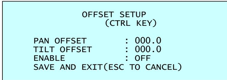
This feature is useful to align a new PTZ camera the same as the previously installed PTZ camera.
