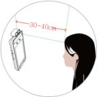
2. To ensure proper and accurate readings, any headgear should be removed so that the sensor can scan the forehead clearly.
