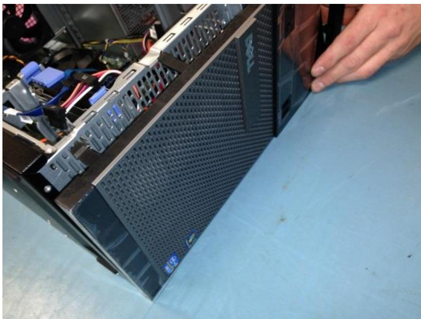
3. Remove the RF Shield (no fasteners involved – should just slide out)
