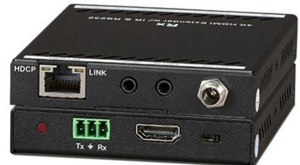
The **KanexPro EXT-HDBT70C** an HDCP 2.2 compliant extender set consisting of a transmitter and receiver. It uses HDBaseT technology to transmit uncompressed, high-resolution 1080p/ 4K signals from transmitter to the receiver via a CAT5e/ CAT6a cable at a distance of up to 70/40m. Moreover, the extender set supports PoC (power over cable) from either side of the sender or receiver, CEC, bi- directional RS232 & IR control.
