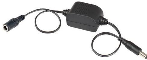
Thank you for your purchase of Speco Technologies' VIDGLT Power Ground Loop Isolator. This unit is especially designed to eliminate the video interference caused when power cable is laid together with video/data cables. It can be easily installed in a new job or added to existing systems. It's useful where a video signal is transmitted via cable between points with different ground potentials. (Difference in ground potentials are typically caused by unbalanced power line loads.)
