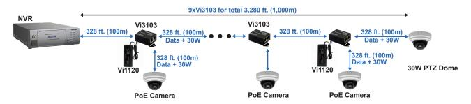
A total of 9 IP addresses can be accessed on a single cable run eliminating the need for network switches.
