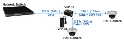
Vi3103 allows for the transmission of two cameras over a single camera run or adding a new camera close to an existing camera.
