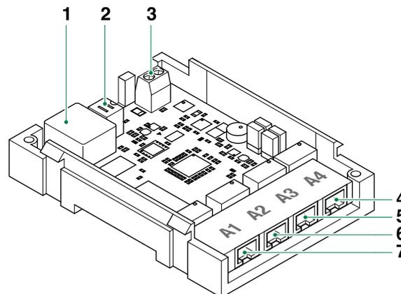
1. **Ethernet port** side B (default: interface not utilised, **Dynamic IP address** 192.168.1.100, subnet mask 255.255.255.0)
