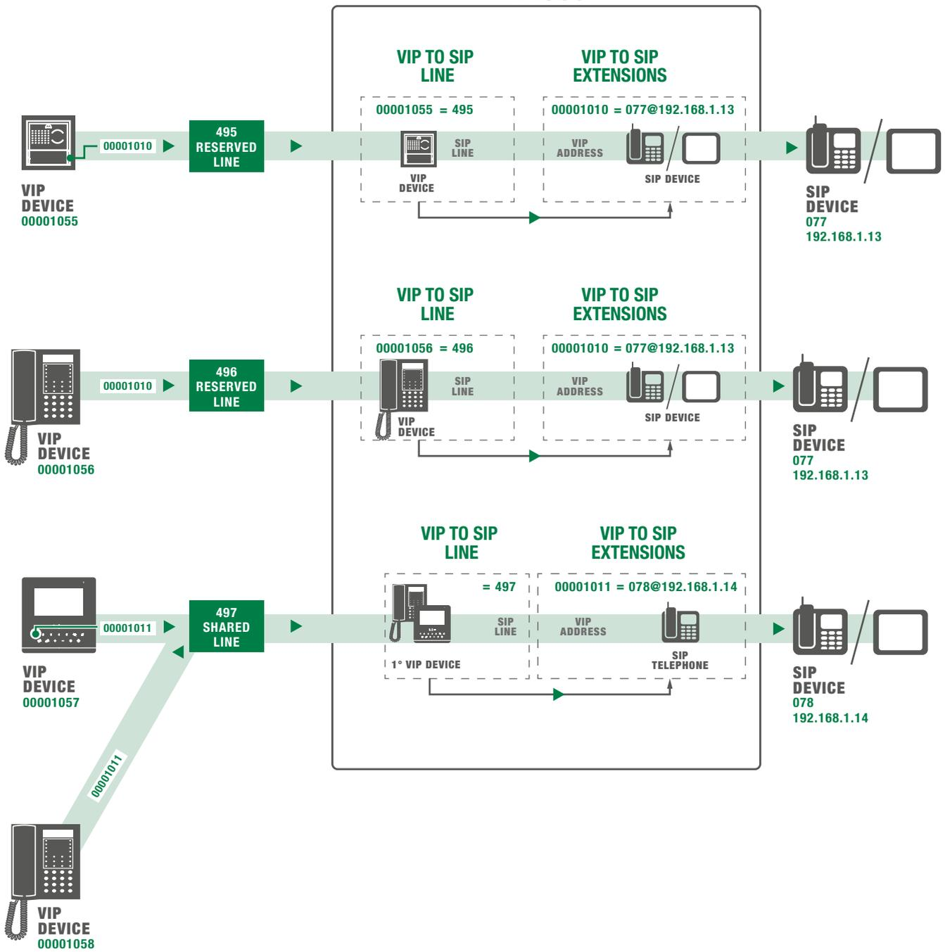
Using a specific command, the SIP devices can call ViP devices associated with reserved SIP lines.
