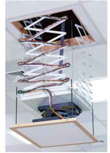
■ Designed for demanding projector applications, the Scissor Lift SL features three sets of scissors to provide lateral and front-to-back projector stability with a maximum 100-pound (45 kg) lifting capacity. The SL offers extension positions for show and service that provide ease of access for projector maintenance. Available with models that vary in maximum lifting capacity and extension to service positions.
